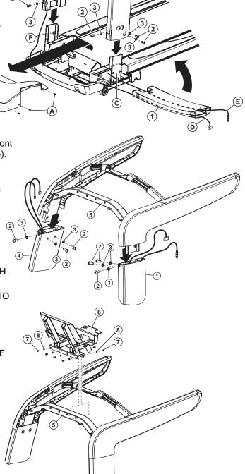
8. Secure the ERGO CROSSBAR of the HANDRAIL/BRIDGE ASSEMBLY (5) to the CONSOLE BRACKET (6) using three SCREWS (31) and three WASHERS (8).
